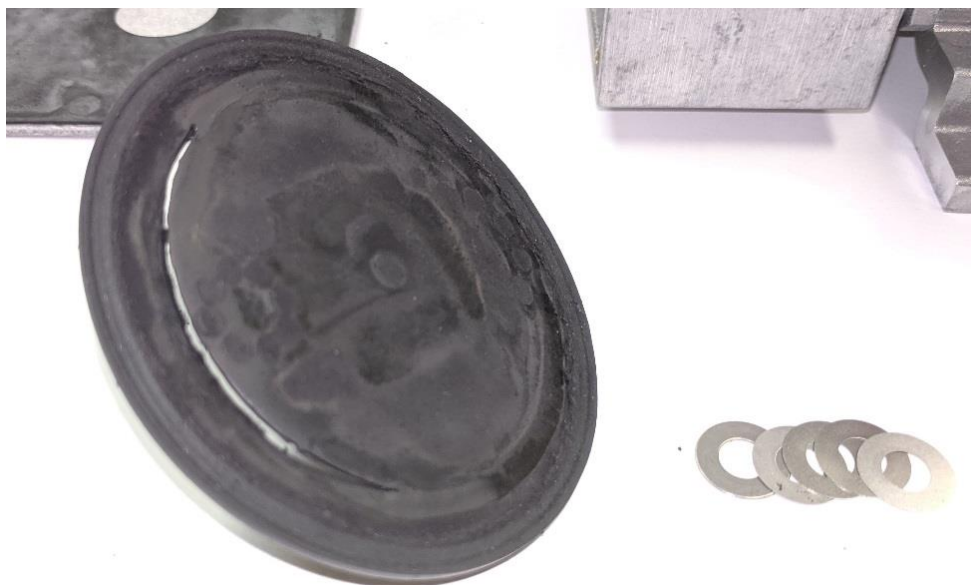
Figure 77: Torn Diaphragm and Diaphragm Spacers
