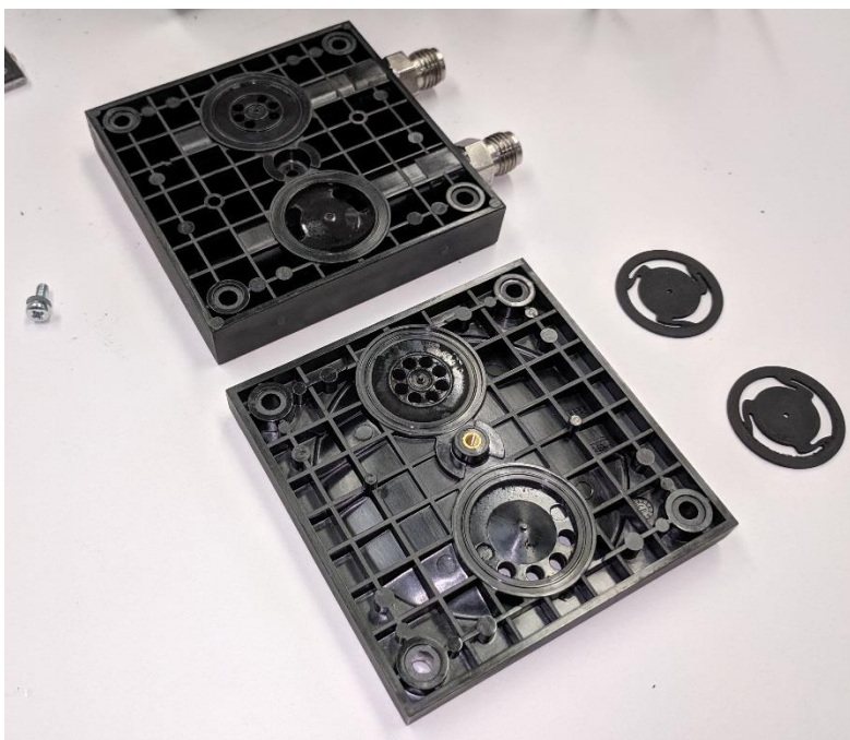
Figure 81: Separated Pump Head Plates with Seals Removed
