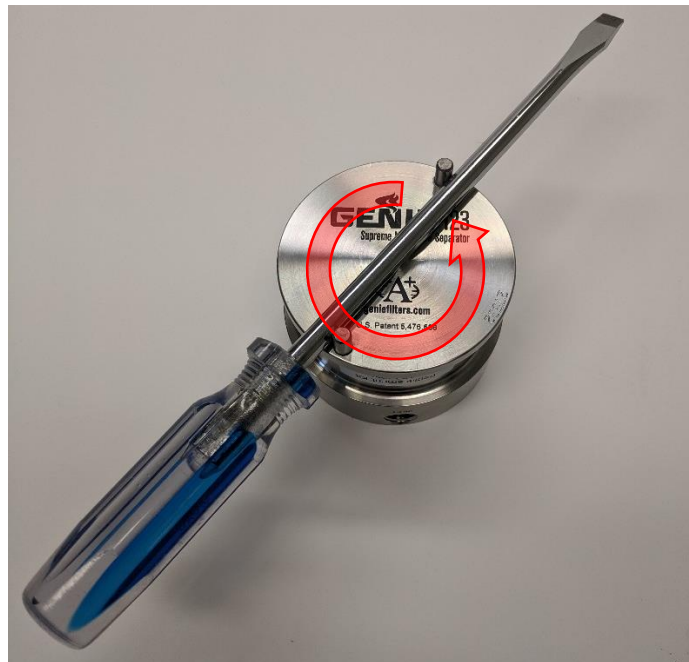
Figure 83: Unscrewing Liquid Membrane Separator Cover with Assistance
