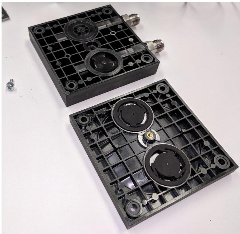
Figure 80: Separated Pump Head Plates
