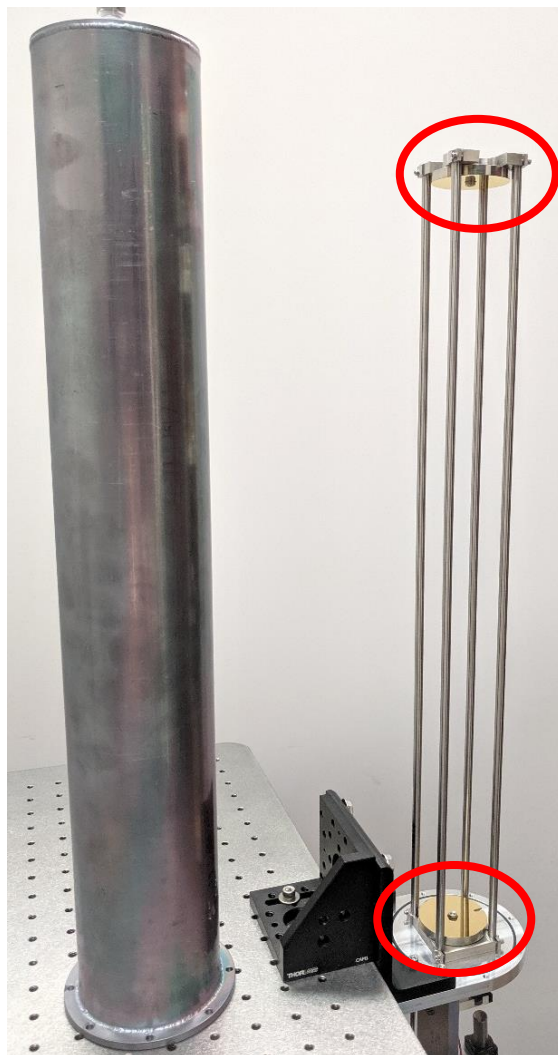
Figure 70: Location of Herriott Cell Mirrors
