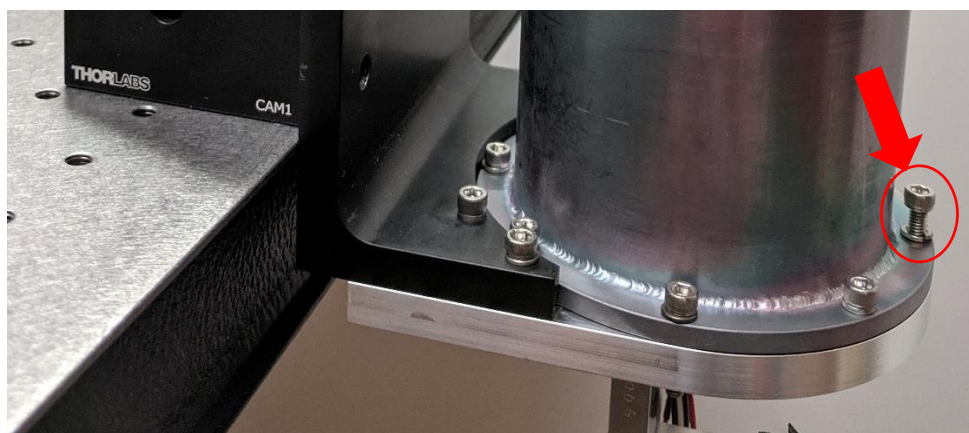
Figure 69: Screws Holding Herriott Cell Cover in Place
