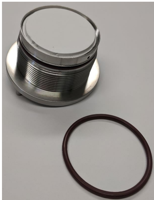
Figure 85: Liquid Membrane Separator Cover with O-ring Removed
